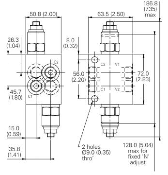
Note: Tightening torque of "F" adjuster locknut= 20-25 Nm.
