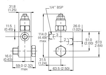
Complete Valve - Gasket Mounted 3/8" Ports Basic Code 1CEG35/1CEBG35/1CERG35/1CELG35 Complete Valve - Dual Overcenter 3/8" Ports Basic Code 1CEE35/1CEEB35/1CEER35/1CEEL35 (Internally Cross-Piloted)
