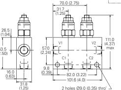
2 holes Ø9.0 (0.35) thro' Where measurements are critical request certified drawings. We reserve the right to change specifications without notice.
